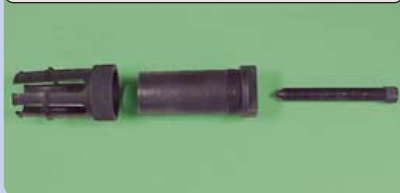
Tool disassembled to show fingers, body and forcing screw
