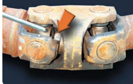
Cardan Joint Cross Yoke Grease Fitting and Needle-Type Applicator
