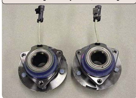
New bearing assembly on left, old on right
