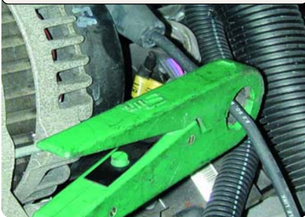
Correct current probe connection at generator
