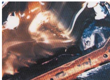
Water in oil, resulting from extreme short-trip driving, photographed through a transparent oil pan.
