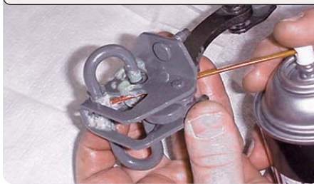
Link removed to show lubrication location
